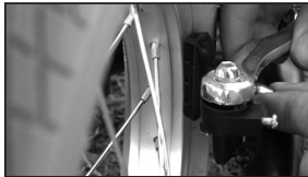
2. Align Brake Shoe to wheel Rim so there is a perfect surface match (both sides)
