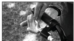
6. Make sure brake handle travel is within 2 fingers when pressed
