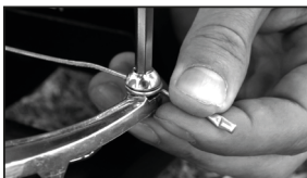
5. Re-adjust the cable by stretching slightly and tighten the bolt
