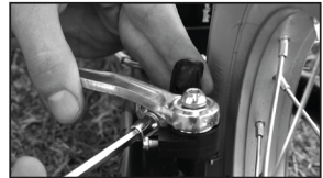
3. Tighten the bolt that secures the brake shoe in position (both sides)
