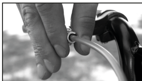
7. If needed adjust the Brake lever travel by turning the cable end screw. Don't forget to lock it with the counter nut.
