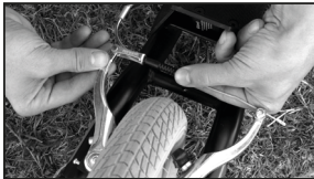
1. Detach the cable end from the slot to open up the Brake arms
